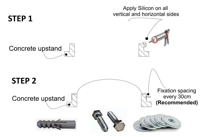
Fisher, Hex. Head Bolt and flat washer for fixation (Recommended)
