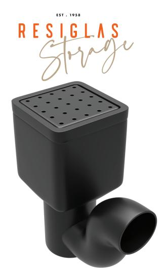
Our Polyethylene Gully Trap is a basin in the ground which receives piped wastewater from your kitchen, bathroom and laundry before it is emptied into the sewer. The gully trap has a water seal to prevent foul odours of the sewer reaching the surface. The top or surround is raised above ground level to prevent stormwater and other foreign matter entering the sewer.
